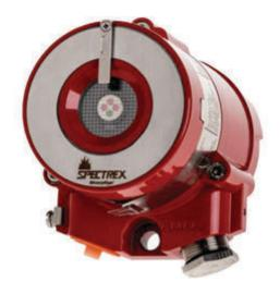
Multi-Spectrum Quad-Sense™ flame detector - integrating four IR sensors to further improve differentiation of flame sources from non-flame background radiation.
